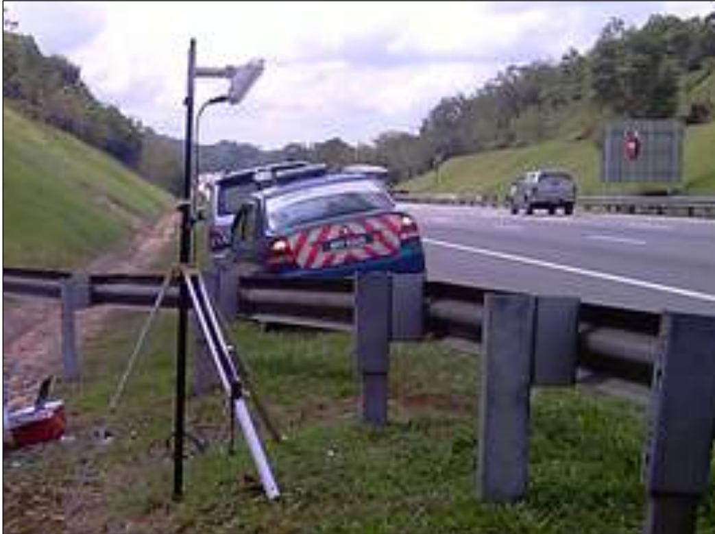
**Figure 1** Smart Sensor used for speed data collection
