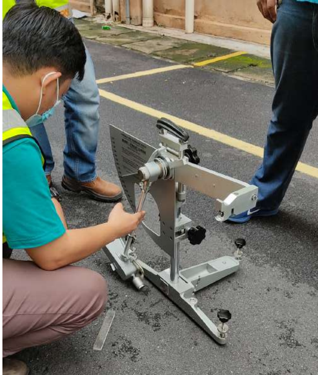
Figure 4 Skid resistance test
