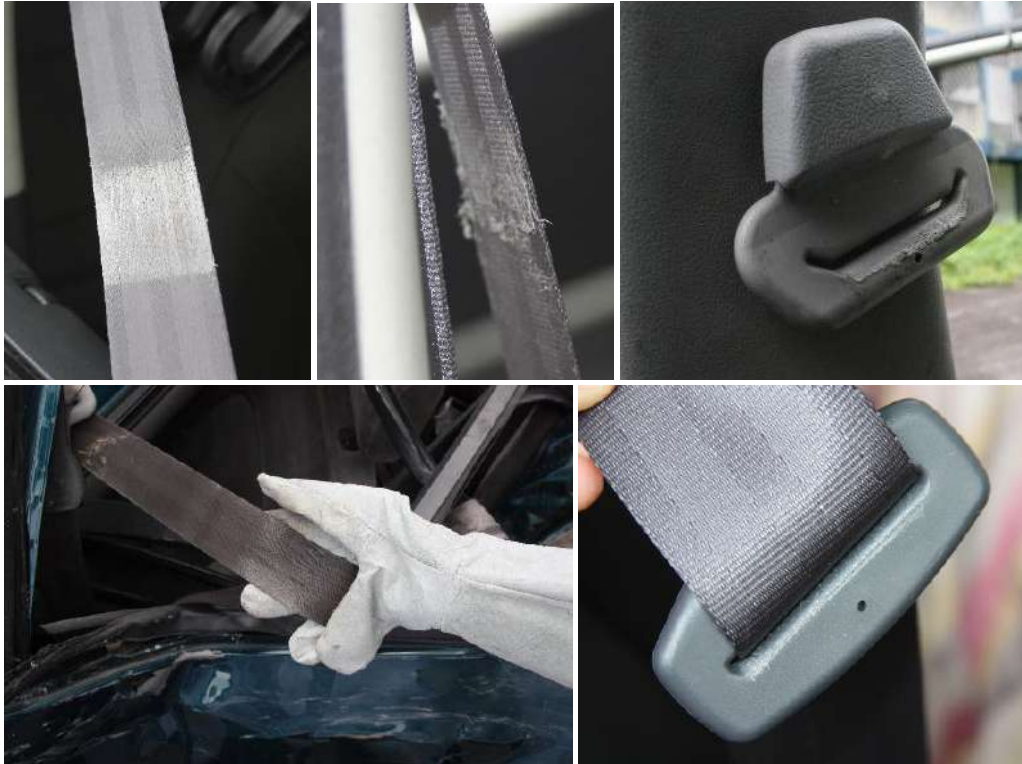
Figure 2 Abrasive marks indicating seatbelt wearing
