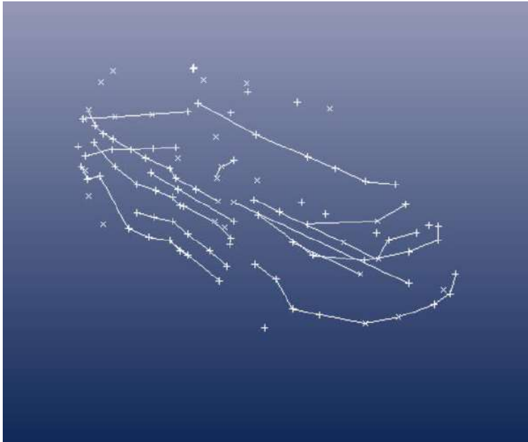
Figure 8 3-dimension points generated with photogrammetry analysis (vehicle 2)
