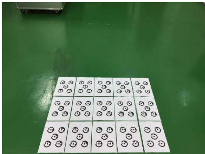
Figure 5 An example of calibration sheet for camera calibration
