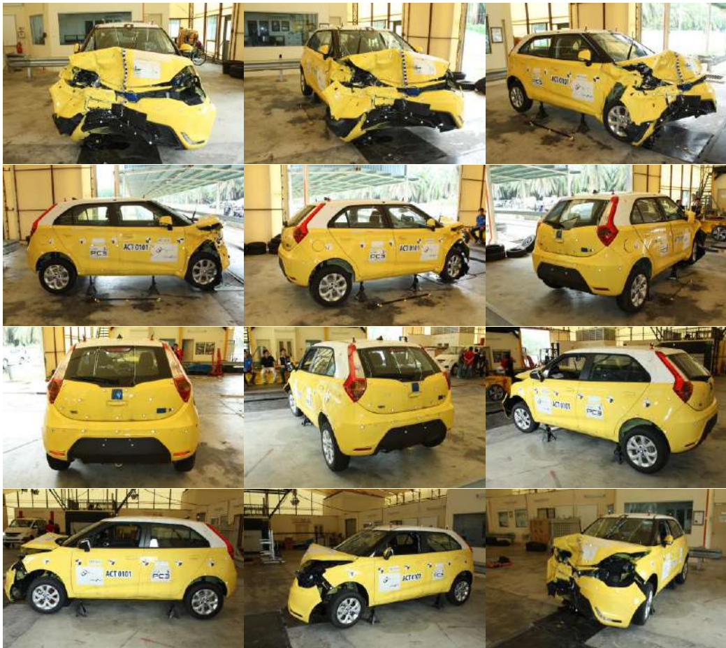
Figure 7 An example of photogrammetry setup for 12-photos set
