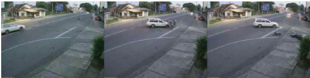
Figure 3 Approach-turn A1 crashes: A turning passenger car failed to see approaching motorcycle from the opposite direction
