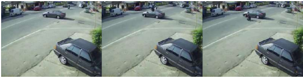
Figure 5 Angle 1A crashes: A right-turn passenger car failed to see travelling straight motorcycle.
