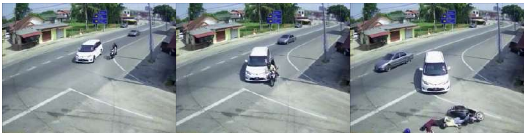
Figure 4 Approach-turn A2 crashes: A turning passenger car failed to see approaching motorcycle from the same direction
