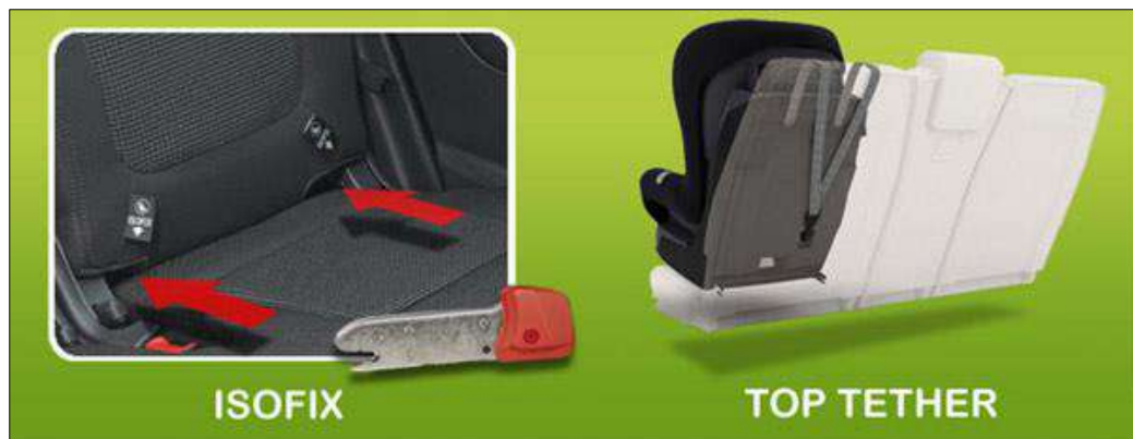
Figure 2 Type of CRS installation
